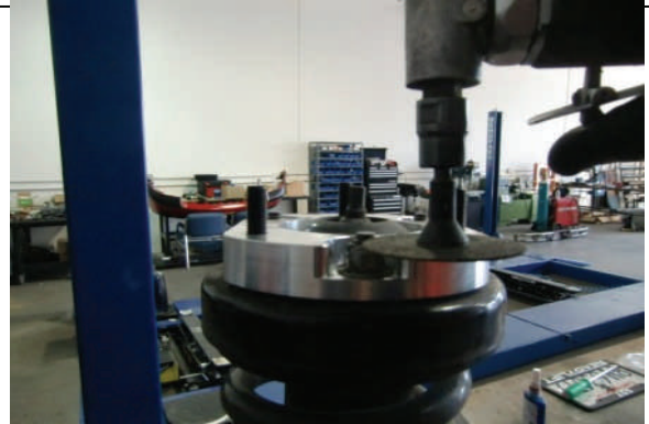
Use cutoff wheel or grinder to trim OE studs flush with spacer
