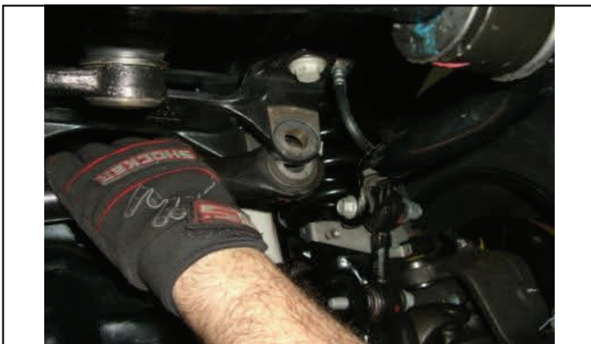
Re-attach track bar to frame mount and torque to spec.
