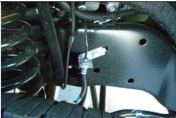
(08-10) models require drilling new 3/8 hole below OE hole.
