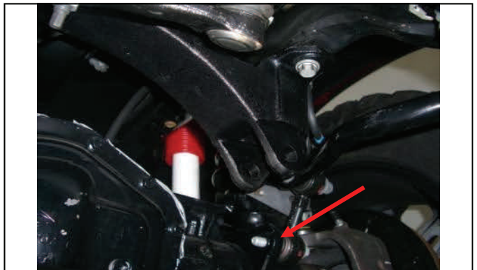
(05-10) Re-attach and tighten sway bar end links.
