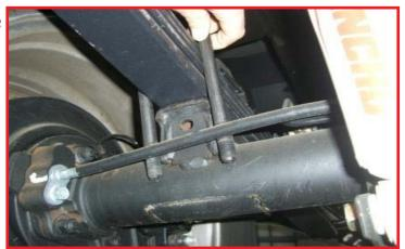
Disconnect the shock from the axle but do not remove it from the vehicle.
