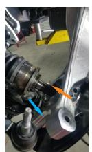
Loosen but do not remove the lower control arm (LCA) hardware at the frame. Lower the LCA while supporting the knuckle and remove the strut from the vehicle. Take care to not over extend or stretch the ABS-rubber brake lines and CV axle. Adjust as necessary.
