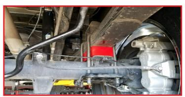
Raise the axle and reconnect the shock to the axle, using the factory hardware. Do not tighten at this time.
