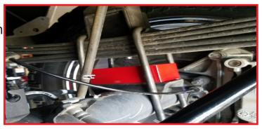
Raise the rear axle until the block is seated between the axle and spring. Install using the provided U-bolts and hardware. Snug but do not fully tighten at this time. Repeat steps for the passenger side.
