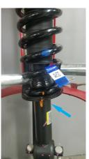
Compress the spring and shock, until the tension is released from the tension nut.
