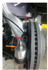
Loosen driver and passenger side sway bar from the frame rails.
