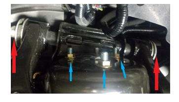
Remove ABS wire from the steering knuckle.
