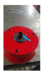
Remove the rubber isolator from the factory top hat. Install the rubber isolator onto the ReadyLift replacement top hat, align the paint mark with one of the studs.
