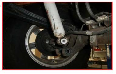
Lower the axle, so the ReadyLIFT rear block will fit between the axle spring perch and the leaf spring, be sure the alignment pins are aligned.
