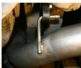
5. With the pipes mounted loosely, adjust the new Flo-Pro system for clearance and appearance. Evenly tighten all clamps starting with the front flange connection working your way to the back.
