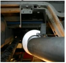
5. Before installing the tailpipe you will need to bolt the supplied hanger to the frame rail.
