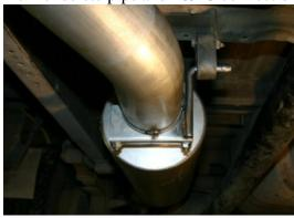
5. Install over-the-axle pipe into outlet of muffler and placing metal hanger into OEM rubber hanger.
