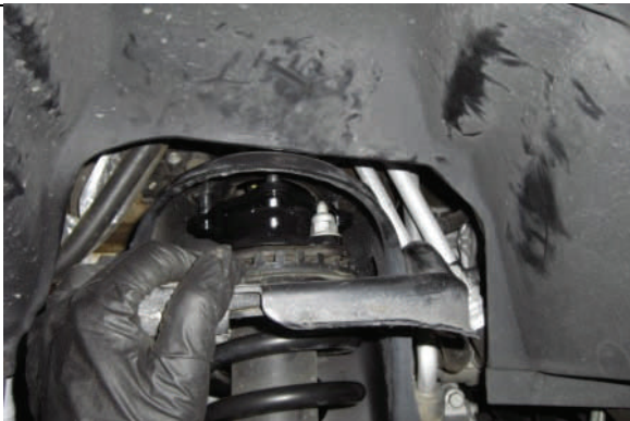
Reinsert strut in chassis and attach with provided hardware
