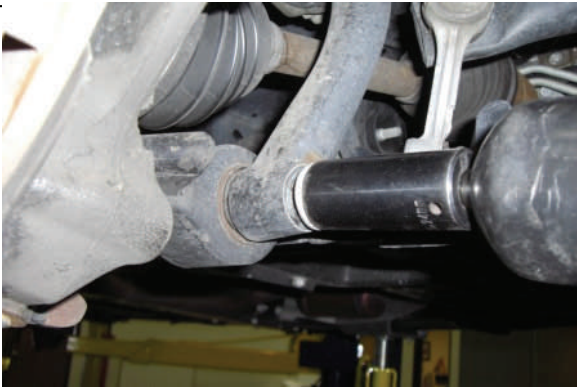
Loosen lower strut mounting nut, leave on
