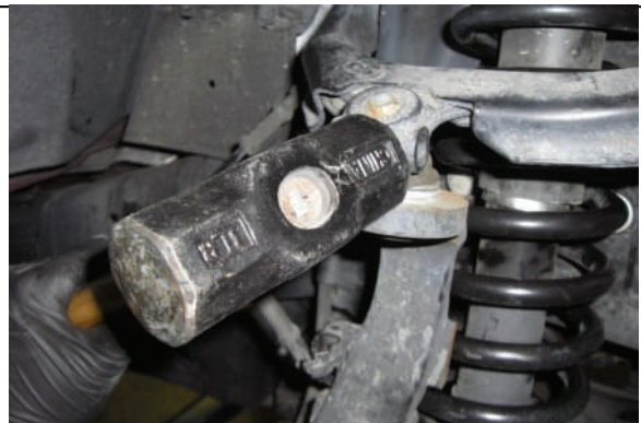
Strike w/ hammer to loosen ball joint from upper control arm
