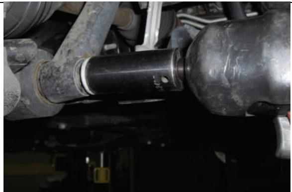
Reattach lower strut mount & sway bar with OE hardware
