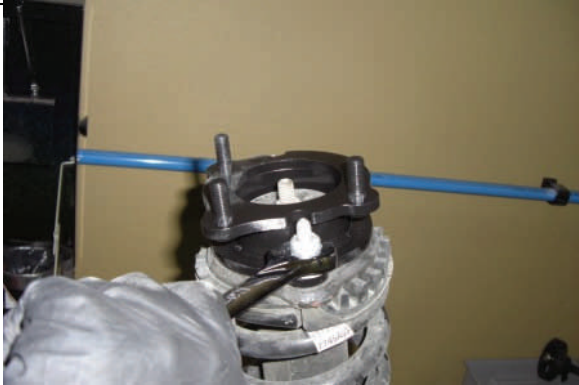
Attach with OE hardware and torque to spec
