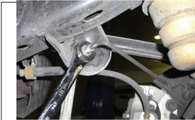
Disconnect rear sway bar end links
