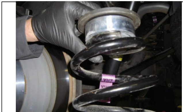
Place new spacer between OE isolator and top of coil spring
