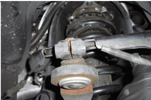
Raise suspension and reattach upper ball joint and torque
