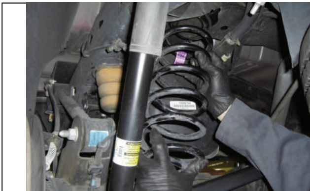
Lower axle slowly and remove rear coil springs
