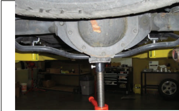
Place jack under rear end to support
