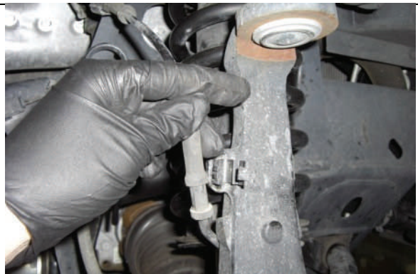
Reconnect ABS wiring to OE clips
