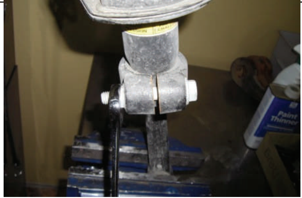
Loosen lower pinch mount on strut and rotate 180 degrees
