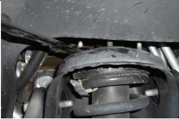
Remove upper strut mounting hardware, remove entire unit
