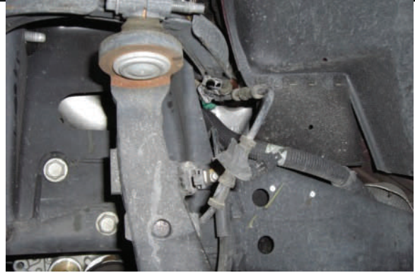
Disconnect ABS wiring at spindle and upper control arm
