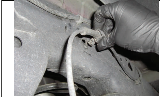
Disconnect ABS wiring at frame to prevent damage
