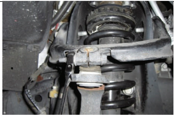
Remove upper ball joint pinch nut
