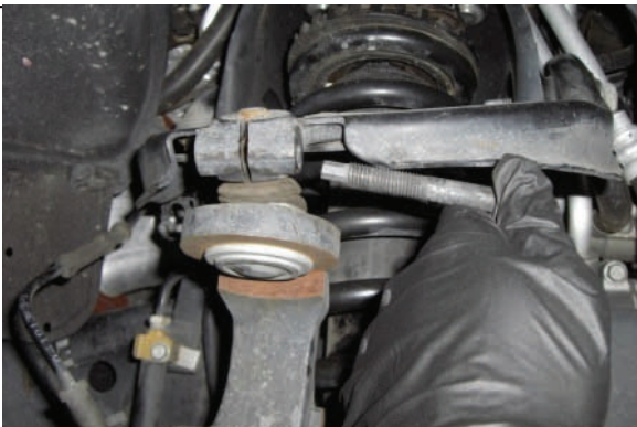
Remove upper ball joint pinch bolt
