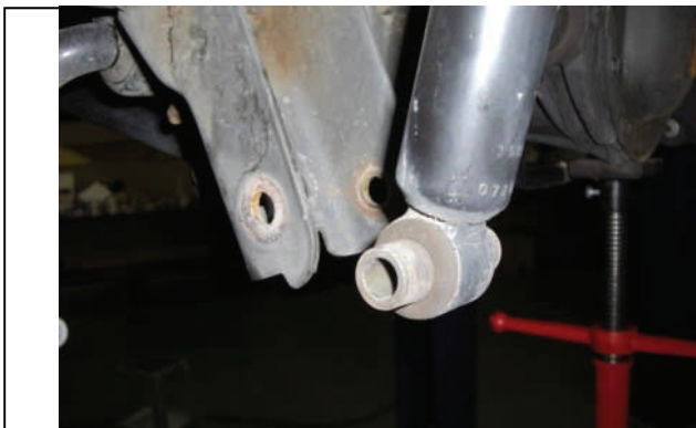
Raise rear suspension and reconnect lower shock, sway bar
