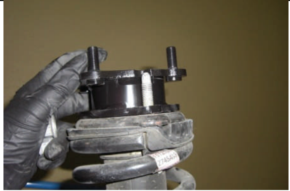
Place strut extension on strut top as shown
