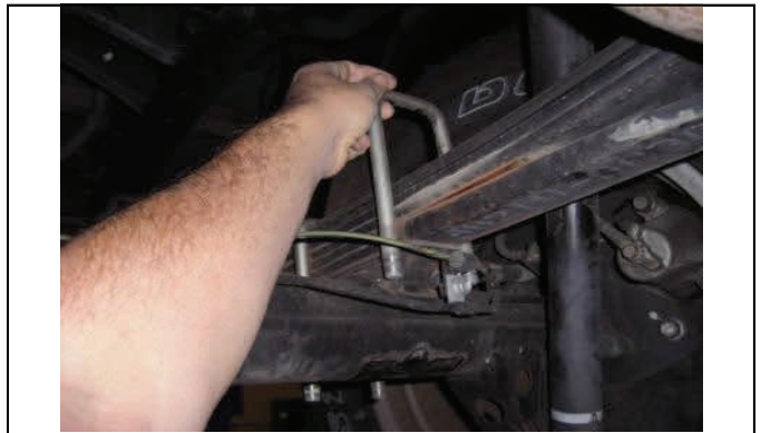
Carefully lower axle and remove u-bolts
