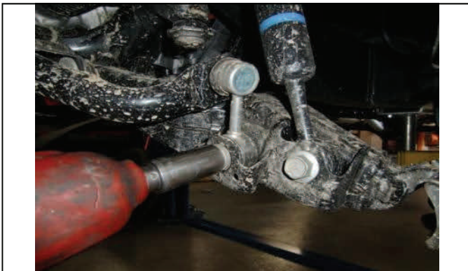
Disconnect lower sway bar end links
