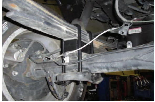
Attach lower mounting plate with provided hardware.
