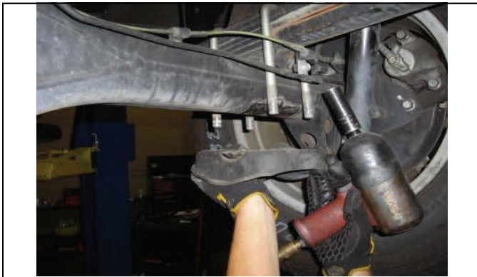
Remove u-bolt nuts and lower plate.
