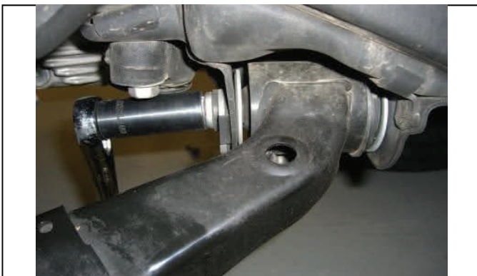
Loosen both lower control arm pivot/alignment bolts
