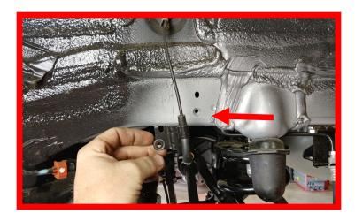
Under the driver side locate the fuel filler shield. Remove the 2 nuts and one plastic rivet. Set cover aside.
