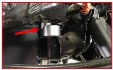
Install the ReadyLIFT ABS drop bracket to the frame using the factory hardware. Install the ABS factory bracket to the drop bracket using the provided 1/4" bolts, washers, and nuts. Torque to 5 ft-lbs.
