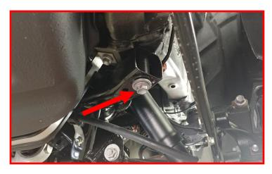
Locate the ReadyLIFT cradle spacers. The round will go in the front location and the square slotted spacers will go in the rear location above the springs.
