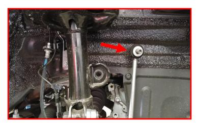
Support the lower control arm with a suitable jack. Remove the two strut to knuckle bolts.
