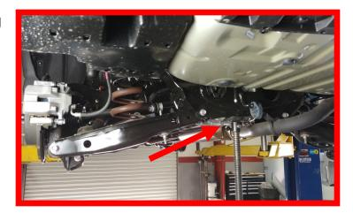
Locate the cradle stud inside the rear spring.
