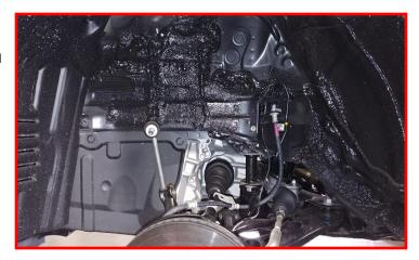
Install the ReadyLIFT strut extensions to the strut using the provided M10 flange nuts. Torque to 30 ft-lbs.
