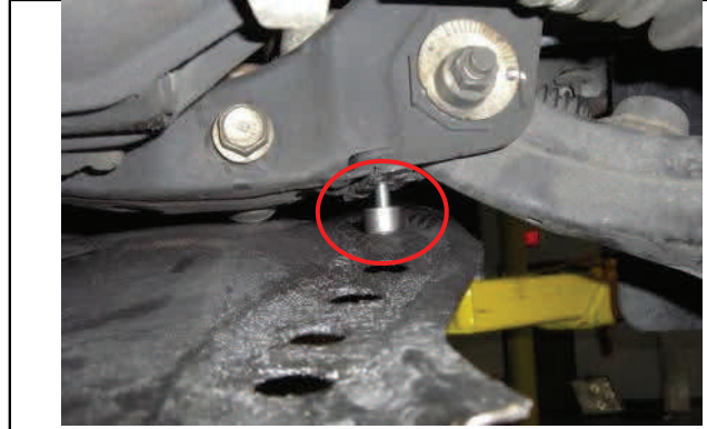
4WD Reattach skid plate with provided spacers and hardware
