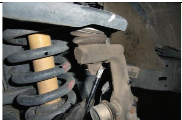
Remove upper ball joint retaining clip
