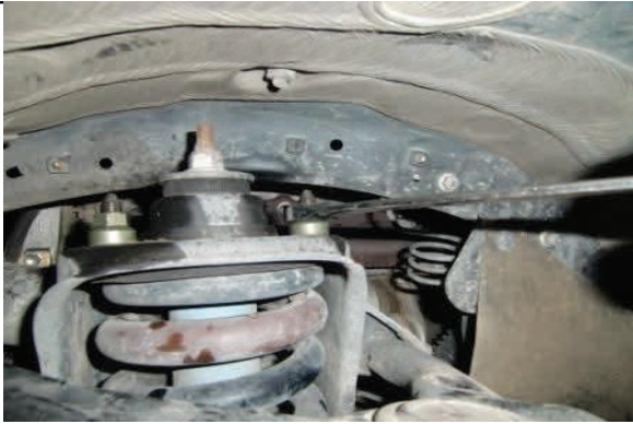
Remove upper strut mounting hardware
