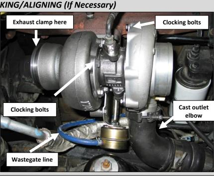
A new compressor outlet O-ring has been provided. Lubricate the O-ring and install between turbo and outlet elbow. Re-use the factory V-Band Clamp. Adjustment of the first intercooler boot may be required for a proper fit.
