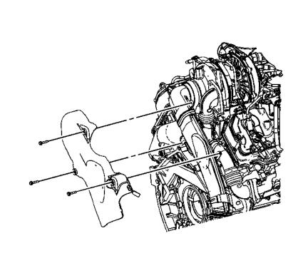
7. Using 12mm 12 point socket wrench remove the passenger side up pipe bolts.
