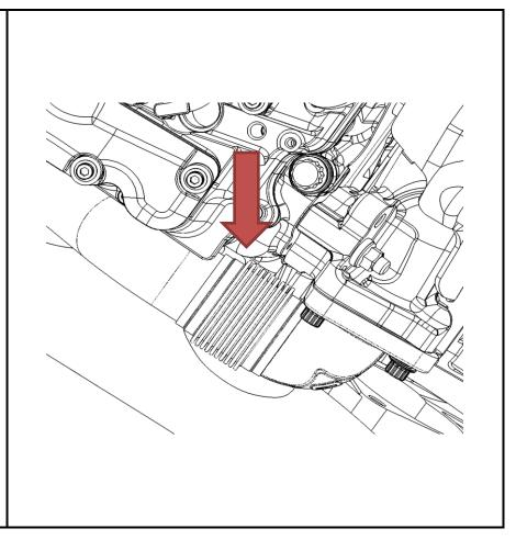
10. Tighten the exhaust up-pipe bolts in the sequence shown. Torque the bolts to 53 Nm (39 lbft)
