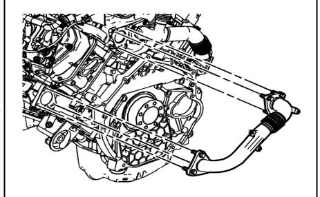
14. Using a plastic scrapper clean the feed port mating surface on the turbo and exhaust manifold.
