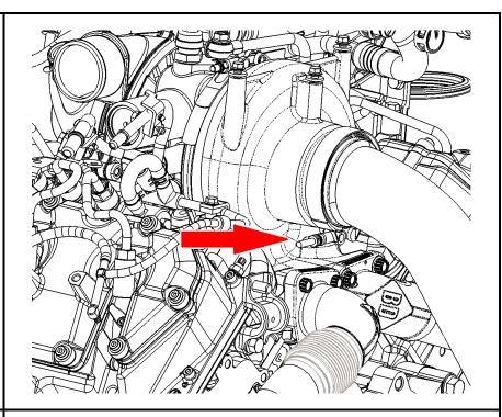
23. Re-install the transmission fluid fill tube. Install fluid fill tube to bellhousing nuts. Torque the nuts to 18 Nm (13 lbft).
