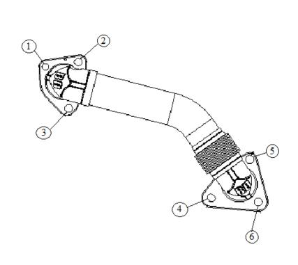
11. To install the driver side up-pipe remove driver side wheel and wheel well.
