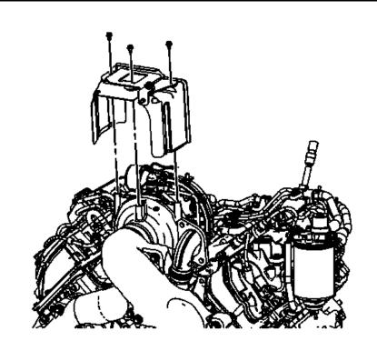
turbocharger 3. Loosen down pipe exhaust turbocharger clamp nut (#1).
