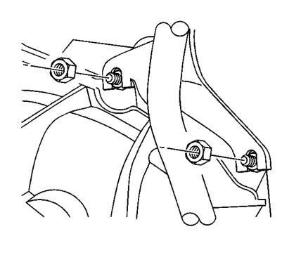
If using an OE/Stock turbocharger exhaust down pipe, remove the heat shield bolts and heat shield.
