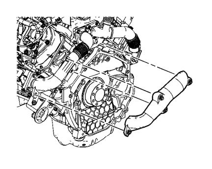
13. Using 12mm 12point socket wrench remove the driver side up pipe bolts.
