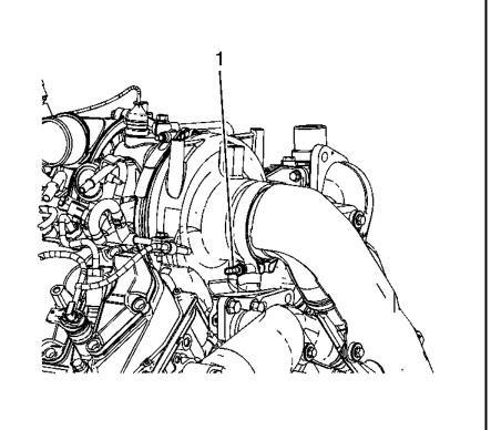
4. Remove turbocharger exhaust pipe to bracket bolt (#1). Remove the turbocharger exhaust pipe. If this is the OEM pipe you will discard as you will need an aftermarket one.
