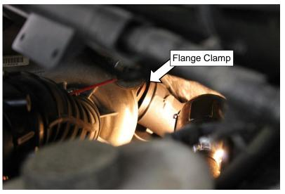
10. Connect the passenger side up pipe to the passenger side exhaust manifold using the supplied hardware. (1900013 & 1900014)
