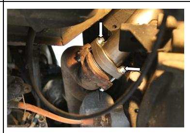
12. Once both pipes are positioned, fully tighten the collector to turbine flange clamp then tighten all pipe connections to 22 ft/lbs.
