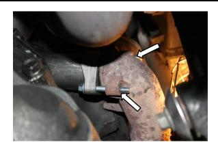
11. Connect the driver's side up pipe to the collector using the supplied gasket and hardware. Then connect the lower connection to the driver's side exhaust manifold with the last two 60mm bolts and nuts (10mm & 12mm).
