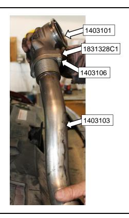
9. Maneuver the pipe assembly into the vehicle and insert the pin on the collector casting into the turbine housing of the turbo. Install the flange clamp (7/16" socket); tighten enough to allow a bit of movement.
