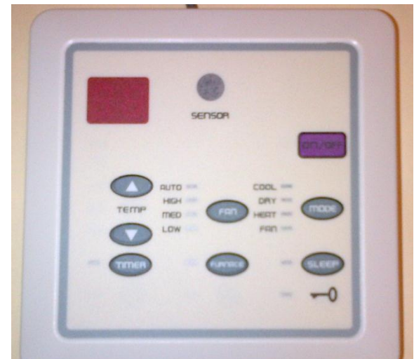
Thermostat control module. A “cool only” model (AC-1351) will not have the furnace pushbutton on the display.
