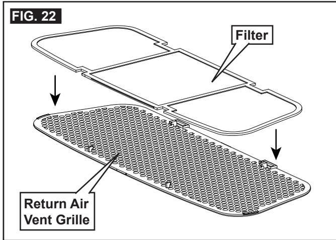
6. Install return air vent grille into the ADB. Slide return air vent grille tab into slot in ADB and rotate up and snap in place. See (FIG. 23).
