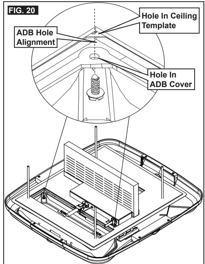
2. Install two (2) (supplied) sheet metal screws inside return air opening to secure ADB to ceiling template. See (FIG. 21).
