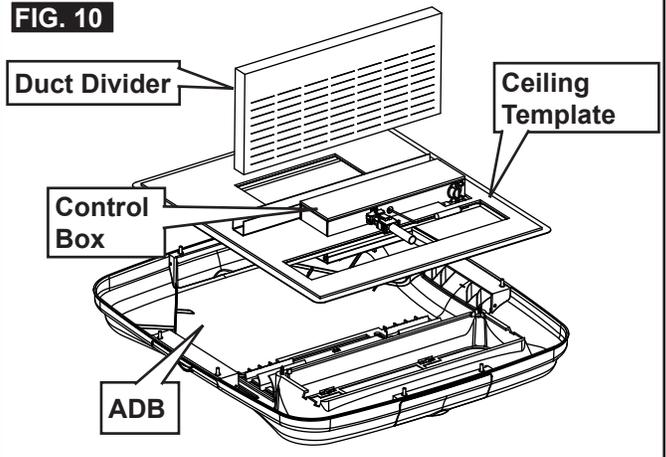
3. All models in this manual will use a four (4) bolt pattern for installing the ADB.
