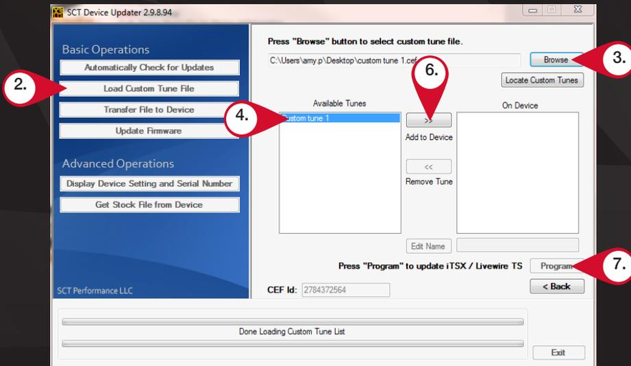
**NOTE:** To edit the name of the file as it appears on your device, you must select the file while it's in the On Device section, type in the desired name in the box below, and click Save.
