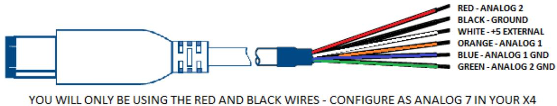
**NOTE:** Do not connect any device that exceeds 5 volts to the analog port or permanent damage to the adapter can occur.
