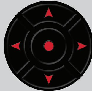
7. While monitoring, **press right or left on the device** to go to the Gauges/Datalog menu. From this menu, you may start recording, select a data log file with which to log, change the gauge layout, and reset the min/max values on the monitor.
