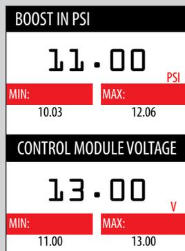
5. The items being monitored can be adjusted by pressing up or down on the device to highlight and then pressing the center button on the X4 to select which reading you'd like to change. Within this menu, you can change the item you're monitoring, and the units in which it will be displaying.
