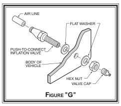
and away from sharp edges. Thermal sleeves have been provided for these conditions. The air line tubing should not be bent or curved sharply as it may buckle. Secure the tubing in place with the nylon ties provided. Push the end of the air line tubing into the inflation valve *see Figure "G"*.
