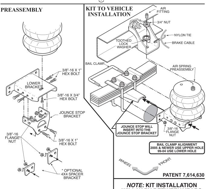
\*NOTE: AN ADDITIONAL SPACER MAY BE NECESSARY FOR SOME 4X4's. IF THE SPACER IS REQUIRED, USE THE SPACER THAT BEST FITS THE VEHICLE.
