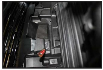
2b. Using a small flat screwdriver, release the two (2) tabs down behind the grille prior to removing the fascia on step 5.
