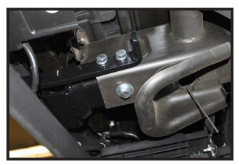
Install the convenience link to the frame with 1/2"-13 x 1-3/4" bolts with 1/2" lock washers. Do this on both sides of the vehicle. Tighten down until the frame squeezes against the baseplate.
