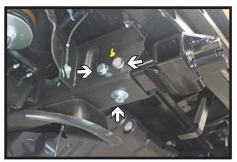
8. Slide the baseplate into the frame pocket and install 1/2"-13 x 1-1/4" bolts with 1/2" lock washers into the outside frame holes and the bottom hole. On the bottom hole use a 1/2" whiz nut on the inside of the frame, using the factory hole for access. Fully tighten all fasteners until the frame squeezes against the baseplate. Do this on both sides of the vehicle.
