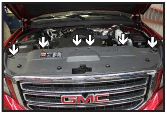
1. Remove the six (6) push pins from the fascia cover and unsnap the front edge. Set the cover aside.
