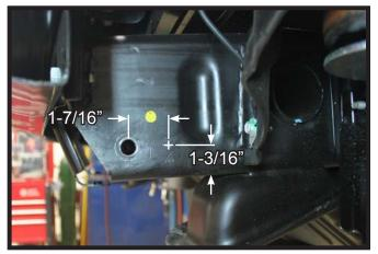
Using a 17/32" drill bit, drill a hole thru the frame 1-7/16" back from the existing hole and 1-3/16" up from the bottom of the frame. Do this on the outside DS frame and the inner PS frame. (DS shown)
