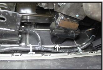
9. Partially reinstall the fascia with a couple of screws along the top and pull the fascia tight against the baseplate. Trace around the attachment tab tube for trimming (Left). Do this on both sides of the vehicle. Remove and trim out the fascia around the attachment tab tubes.
