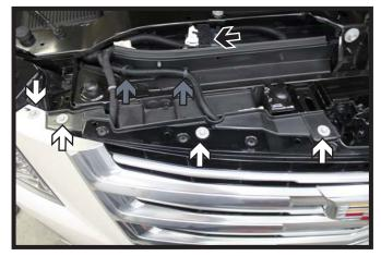
2a. Using a 10MM socket, remove the eight (8) screws from the top edge of the fascia. There are four (4) on each side.On the passenger side only, disconnect the plug (black) and remove the two (2) clips holding the wiring loom (gray).
