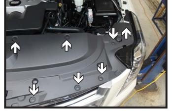
1. Remove the fourteen (14) push pins from the fascia cover and set aside. There are seven (7) on each side.
