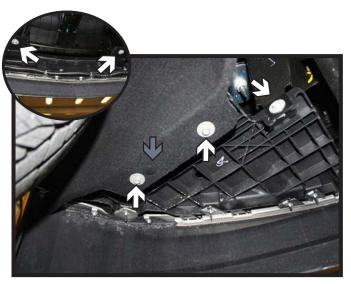
Using a 10MM socket, remove the eight (8) screws from the underside of the fascia. There are three (3) on each side and two (2) in the middle. Remove the two (2) push pins located in front of the tires (gray).
