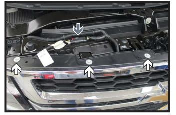
Using a 10MM socket, remove the six (6) screws from the top edge of the fascia (white). There are three (3) on each side. On the passenger side, disconnect the wiring harness (gray).
