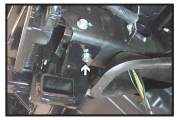
8. Using a 17/32" drill bit, drill out the existing hole in the bottom of the frame. Install a 1/2"-13 x 1-1/2" bolt with lock washer into the hole and a 1/2"-13 whiz nut on the inside of the frame. Do this on both sides of the vehicle. Fully tighten all hardware.
