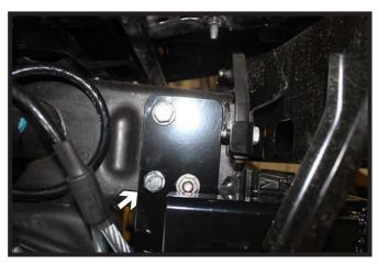
10. On the driver side, install 1/2"-13 x 1-1/2" bolt with lock washer into the hole and a 1/2"-13 whiz nut on the inside of the frame. Fully tighten all hardware.
