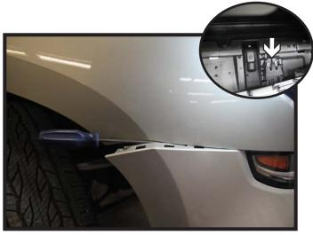
5. Gently pry the clips of the corners of the fascia loose from the fender. Behind the grille towards the base, pop loose the two (2) clips. Remove the fascia from the vehicle and set aside.
