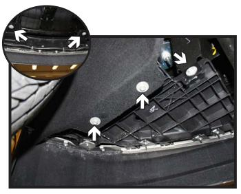
Using a 10MM socket, remove the eight (8) screws from the underside of the fascia. There are three (3) on each side and two (2) in the middle.
