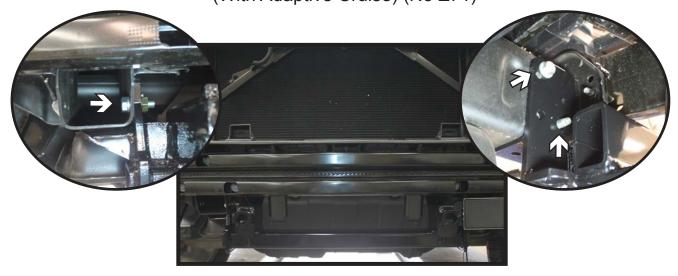
7. Align the baseplate to the existing holes in the frame. Start the two (2) existing bolts on the driver side that were removed from the ACC bracket (right). On the passenger side install a 1/2"-13 x 1-1/2" bolt with lock washer into the existing hole and a 1/2"-13 whiz nut on the inside (left). Level the baseplate and fully tighten all hardware.
