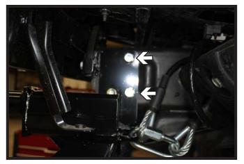
Using a 17/32" drill bit, drill out the remaining holes in the inside of the passenger side frame. Install 1/2"-13 x 1-1/2" bolts with lock washers into the hole and a 1/2"-13 whiz nuts on the inside of the frame. Fully tighten all hardware.
