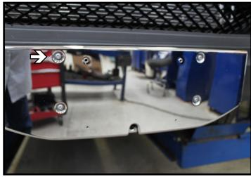
6. Using a 20 Torx remove the four (4) bolts and remove the license plate bracket.
