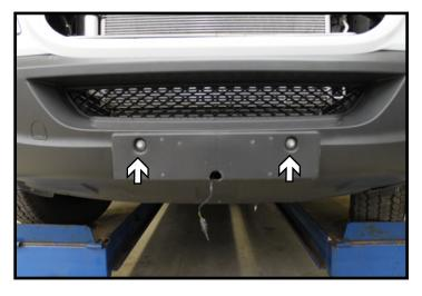
7. Remove the two (2) bolts using a 13mm socket, then remove front facia.
