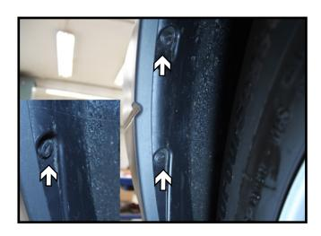
In the front wheel well using a straight screwdriver, turn the two (2) upper and one (1) lower facia pins 90 degrees to unlock and remove. Both driver and passenger sides.
