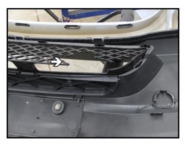
17. Hold front facia up to frame and mark to cut out for clearance around baseplate. After cutting sufficient amount for clearance, reattach facia to vehicle.
