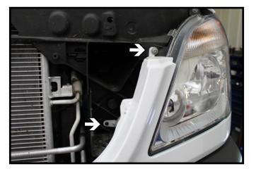
4. Remove the upper screw using a 27 Torx and lower screw using a 20 Torx on both driver and passenger sides.
