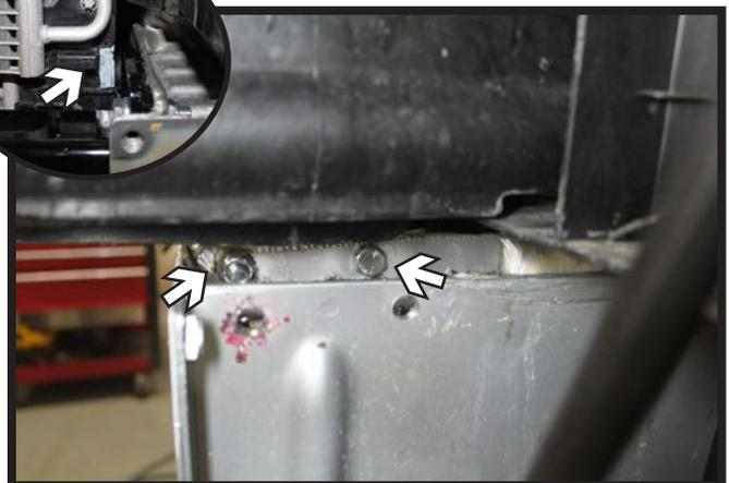
13. Using a 3/8" drill bit, drill thru the frame lips into the top baseplate holes. Install the 3/8" hardware into the top holes and fully tighten. Do this on both sides of the vehicle. Note: the plastic shielding behind may need to be trimmed for easier nut access (inset).
