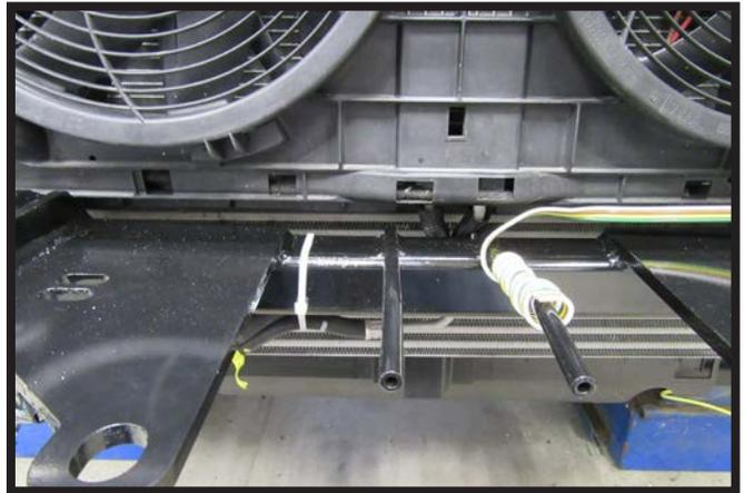
15. Install the wire loom cover around the condenser lines to prevent rubbing (left). And zip-tie the line to the baseplate to prevent it from moving around (right).
