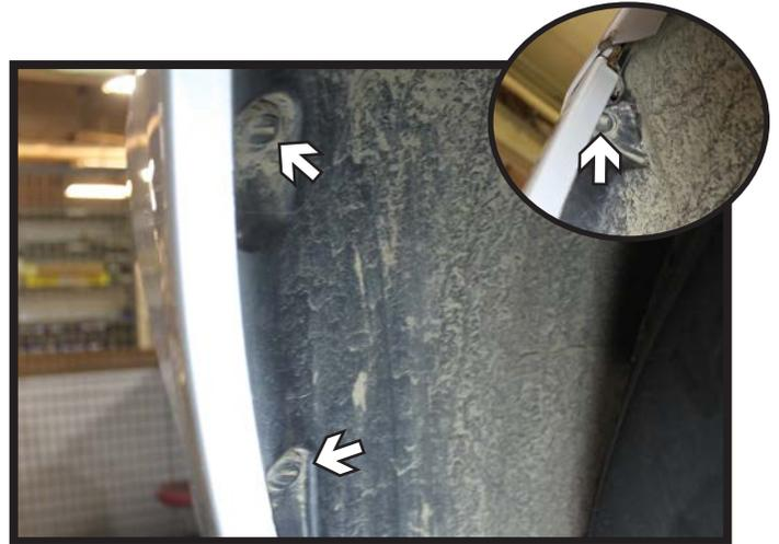
2. Remove the three (3) push pins in the wheel well. Do this on both sides of the vehicle.
