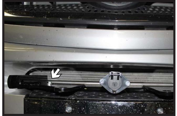
17. Reinstall the bumper. Reinstall the fascia with the 3/4" spacers in the step area bolt recess areas (left). After the fascia is on the vehicle, install the 8MM hardware thru the baseplate into the step area bolt areas and fully tighten.
