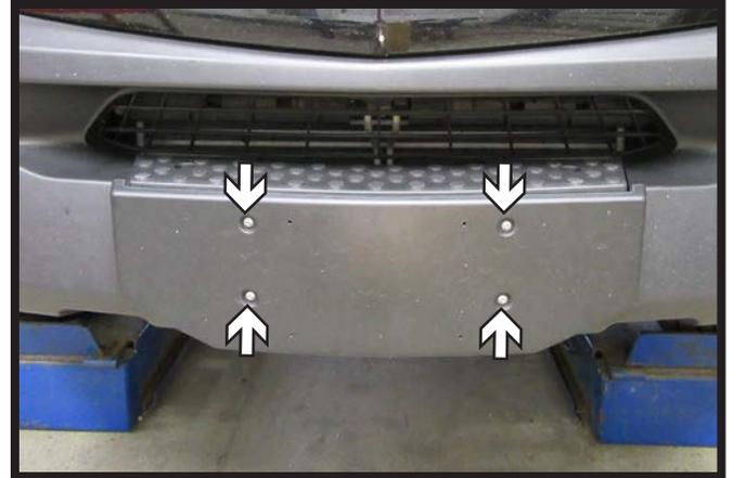
4. Using a T20 Torx, remove the four (4) screws from the front cover.
