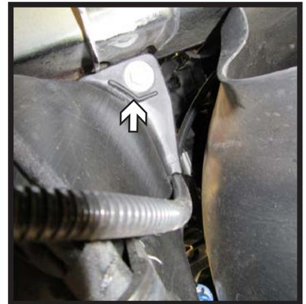
10. On the passenger side, using a 18MM socket, remove the front bolt (middle) from the tank. Then using a 13MM socket, remove the rear bolt (right) and let the tank hang down.
