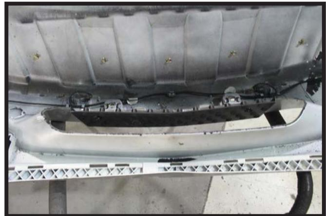
16. On the back side of the fascia, trim off the inner grille at the joint all the way around.
