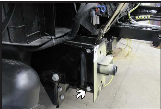
12. Clamp the baseplate to the frame of the vehicle. Using a 3/8" drill bit, drill the lower front baseplate hole thru the frame. Install the 3/8" hardware into the hole and fully tighten. Do this on both sides of the vehicle.
