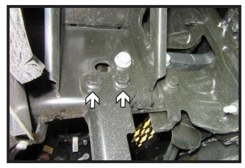
Using a 24MM socket, remove the two
