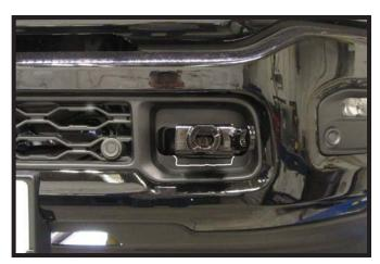
Slide baseplate into tow hook housing as far as possible. Mark plastic for trimming. Do this on both sides of the vehicle.
