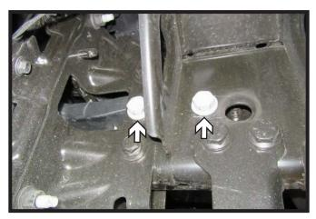
1. Using a 24MM socket, remove the two (2) bolts from the tow hook. Do this on both sides of the vehicle.
