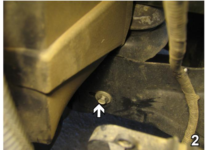
2. Just behind the metal bumper on the frame down by the headlight, there is a bolt that needs to be removed. Use a 15MM socket. Do this to both sides. Set bolts aside to be reinstalled later.
