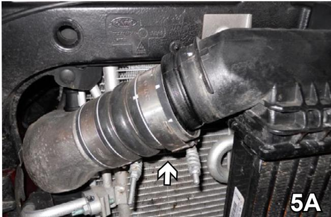
5. Models with Turbo cooler will need to loosen and disconnect both clamps, then carefully set cooler aside. Cooler will be reinstalled later.
