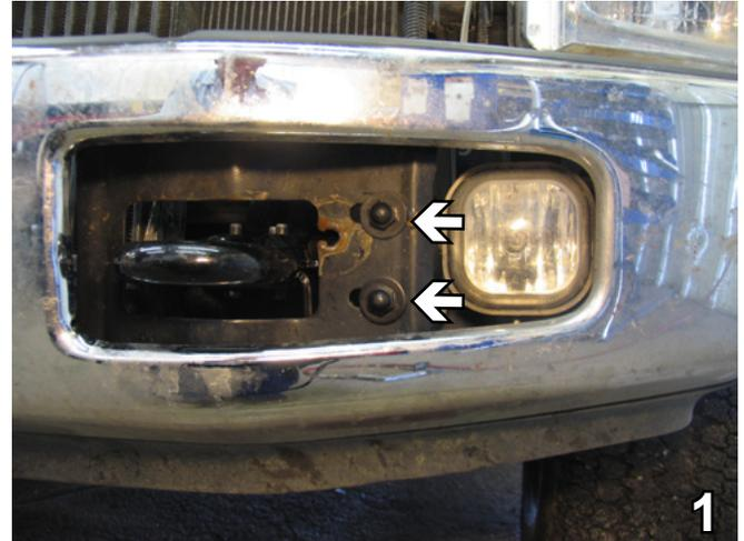
1. Using a 18MM socket, remove two metric bolts from the bumper, located just beside the fog light assembly. Do this to both sides of the vehicle. Set bolts aside to be reinstalled later.
