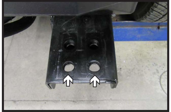
9. Remove the two (2) bolts from each side of the bracket near the tow hook by using an 18MM socket. Do this on both sides of the vehicle.
