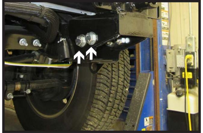
12. Use three (3) 1-3/4" bolts to attach the baseplate towards the outside of the frame. Use a flat washer on the outside and nylon lock nut on the inside for the front two (2) bolts indicated with a white arrows and a flat washer and nylon lock nut on the inside for the third bolt indicated with a gray arrow. Towards the inside of the frame use two (2) 1-3/4" bolts to attach the baseplate with the washer on the outside and nylon lock nut on the inside. Do this on both sides of the vehicle.
