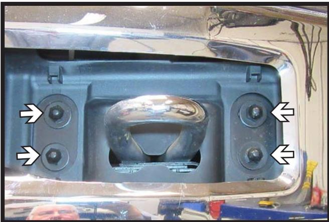
7. Using a 18MM socket, remove the four (4) bolts around the tow hook. Do this on both sides of the vehicle. Pull the bumper forward and set aside to be reinstalled later.
