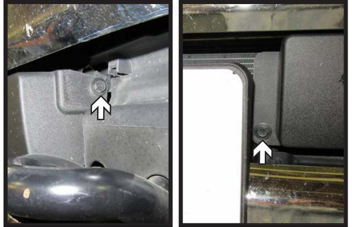
4. **Models with Adaptive Cruise Control (ACC):** Using a 10MM socket, remove the two (2) bolts from the cover of the ACC on the driver side of the vehicle.
