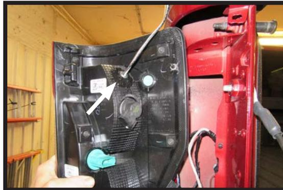
Drill a hole according to the tail
