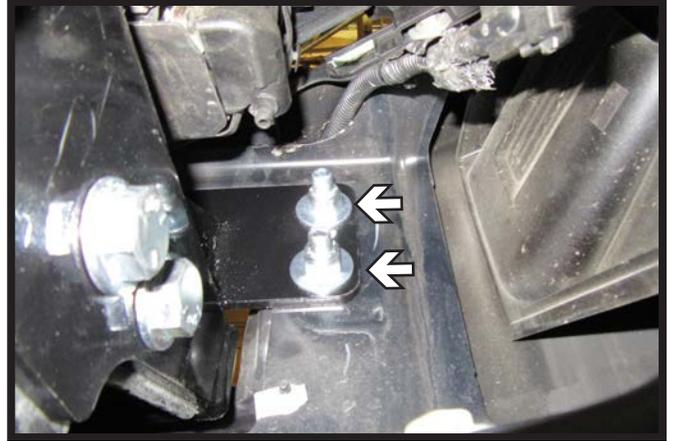
17. Insert two (2) 1/2" x 2" bolts with a flat washer and nylon lock nut on the back side to attach the convenience link. Do this on both sides of the vehicle.
