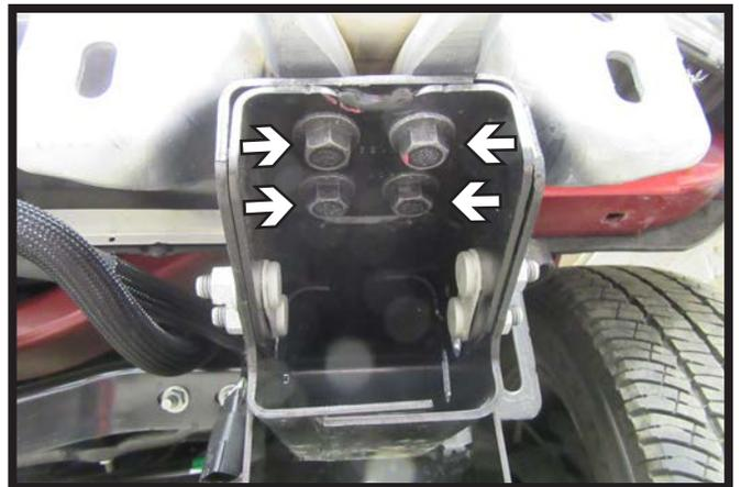
8. Using an 18MM socket, remove the four (4) bolts from the bottom of the tow hooks on both sides of the vehicle.
