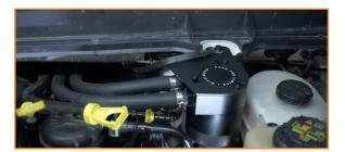
30. Reinstall the hot-side intercooler pipe.(1x worm gear clamps, 1x spring clip)
