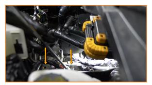
Remove the bolts that secure the air-oil separator. (4x 8mm bolts)
