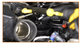
Remove the bolts that secure the fuel rail. (2x 8mm bolts)
