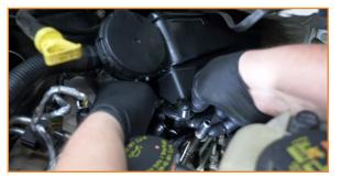
10. Lubricate the new O-ring and install the Mishimoto adapter to the bottom of the air-oil separator.
