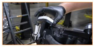
Install the three long bolts provided with the aluminum adapters. Leave the bolts loose for now. (3x 10mm bolts) 18. Install the small aluminum bracket between the valve cover and the air-oil separator.(1x 10mm bolt, 1x 5mm Allen bolt)
