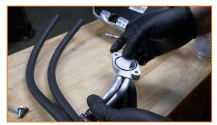
16. Install the adapter and hoses to the back end of the air-oil separator. Make sure the O-ring has not fallen off the bottom of the adapter. The image below was taken with the separator out of the vehicle for a clearer representation.
