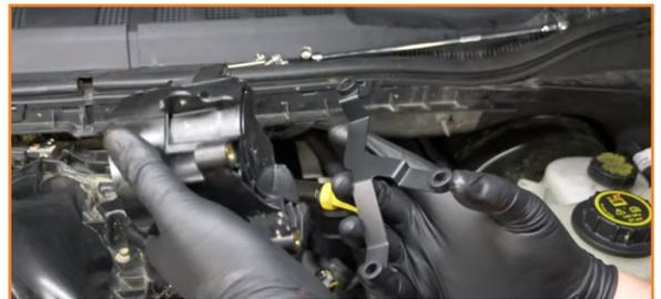
24. Reinstall the fuel filter bracket along with the Mishimoto bracket using the three provided long bolts and one short bolt. Torque the three long bolts to 89\_in./lb. (10nm.). (3x 8mm long bolts, 1x 8mm short bolt)
