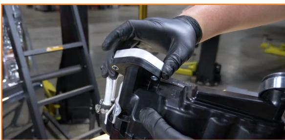
19. Install the three long bolts provided with the aluminum adapters. Leave the bolts loose for now. (3x 10mm bolts)
