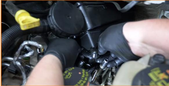
17. Lubricate the new O-ring and install the Mishimoto adapter to the bottom of the air-oil separator.
