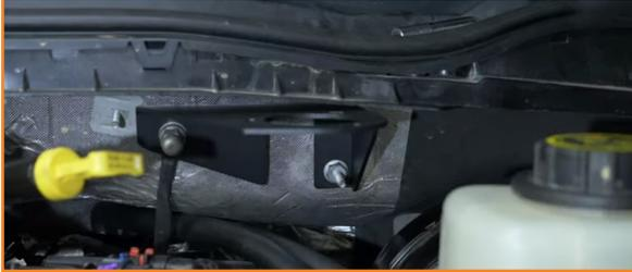
29. Thread the fittings onto the catch can. Tighten the fittings with a wrench.
