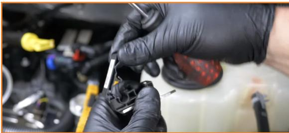
9. Replace the stock metal bracket attached to the fuel line retaining clip with the provided Mishimoto bracket.
