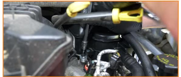
21. Torque the three previously installed long bolts to 89\_in./lb. (10nm.). (3x10mm bolts)
