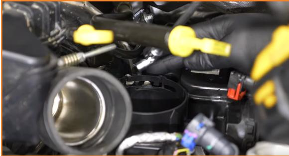
6. Remove the bolts that secure the fuel rail. (2x 8mm bolts)
