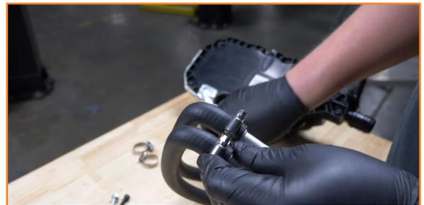
14. Grease the O-ring groove on the aluminum adapter and place the thin O-ring within the groove. This was done outside the vehicle for a clear representation.
