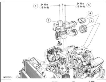
4. Remove the Charge Air Cooler tube.
