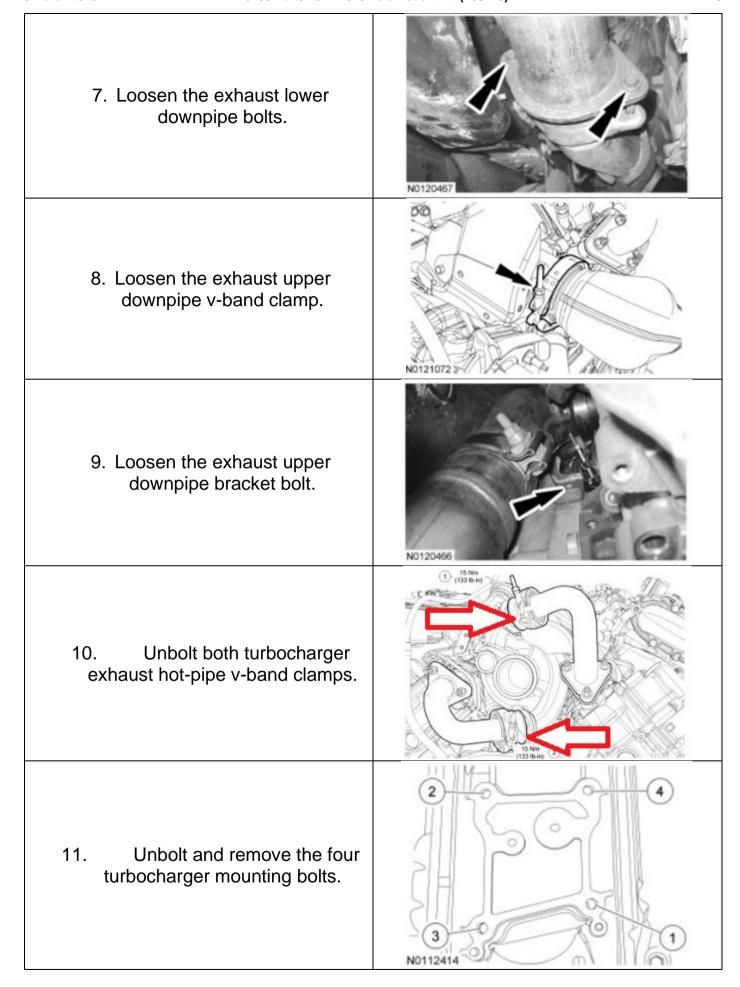
Remove turbocharger.Keep OEM heat shield.
