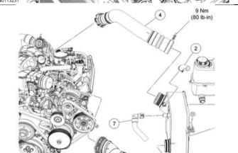
5. Disconnect the turbocharger actuator electrical connector and disconnect the wastegate actuator vacuum hose on pickup models.
