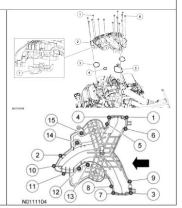
3. Remove the lower intake manifold.
