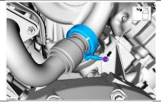
Connect turbocharger downpipe v-band clamp, and downpipe bracket bolt.
