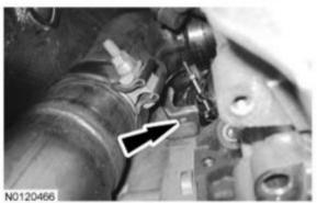
9. Re-install the lower exhaust downpipe bolts and torque to 26 lb ft (35 Nm).
