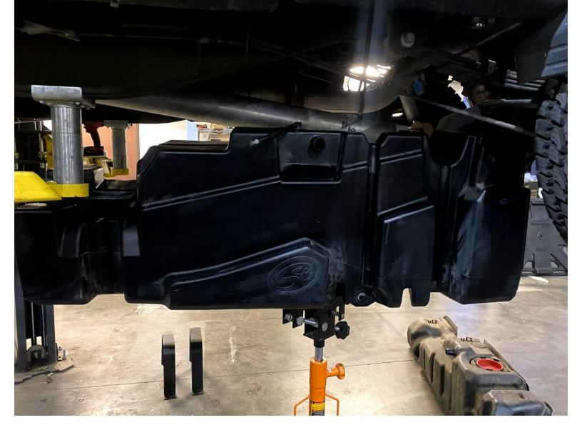
Place the tank onto the transmission jack and lift the tank into place. The tank will need to be angled over the driveshaft. The driveshaft can be disconnected from the rear axle and held away from the tank to make this easier.
