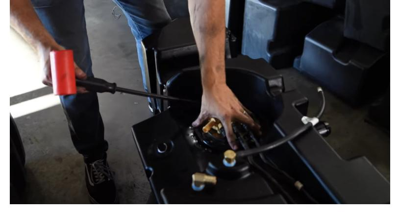
Place the retaining ring over the sending unit and push down to get the ring started under the receiving teeth on the S&B Tank. With a pry bar and mallet, hit the ring clockwise until the ring is fully rotated under the indention.
