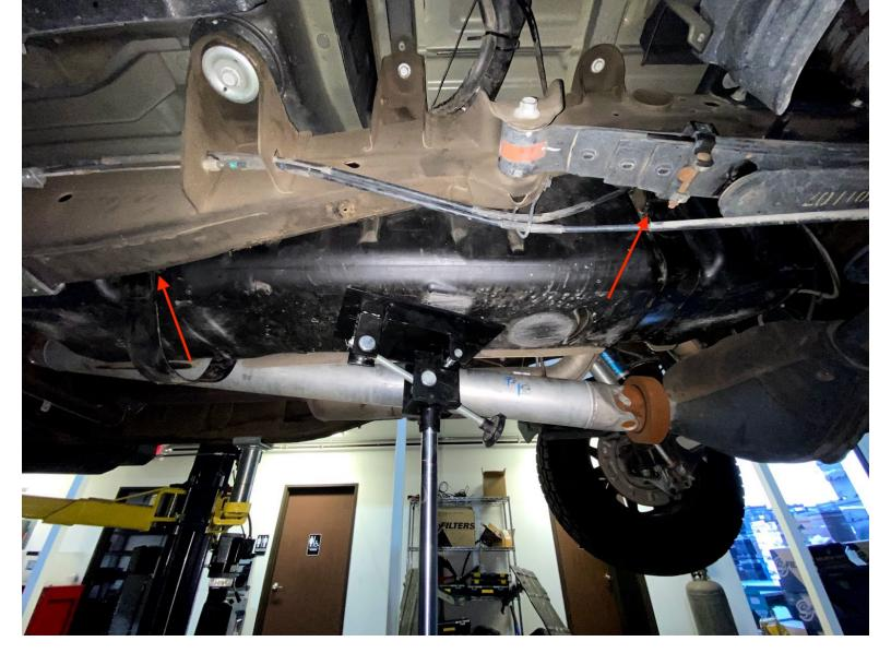
Remove the 2 bolts that secure the fuel tank straps and then lift our the strap on the driveline side.
