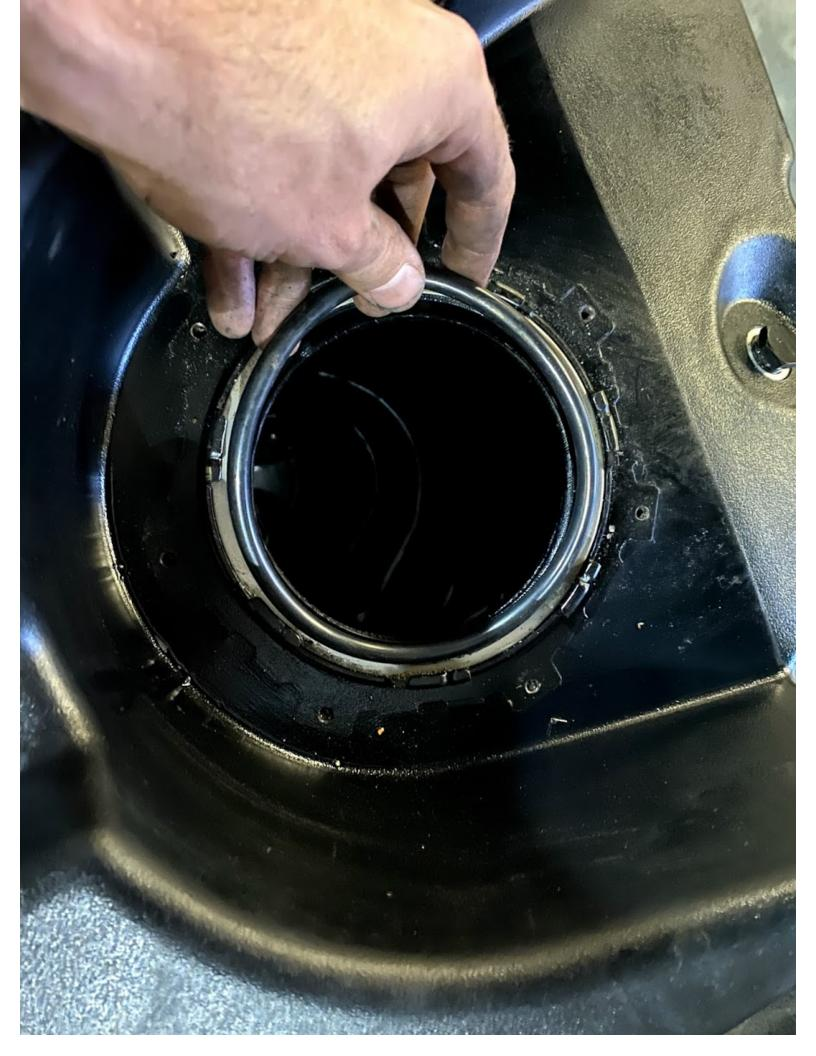
Check the inside of the tank to make sure there are no foreign debris. Place the o-ring in the o-ring groove.
