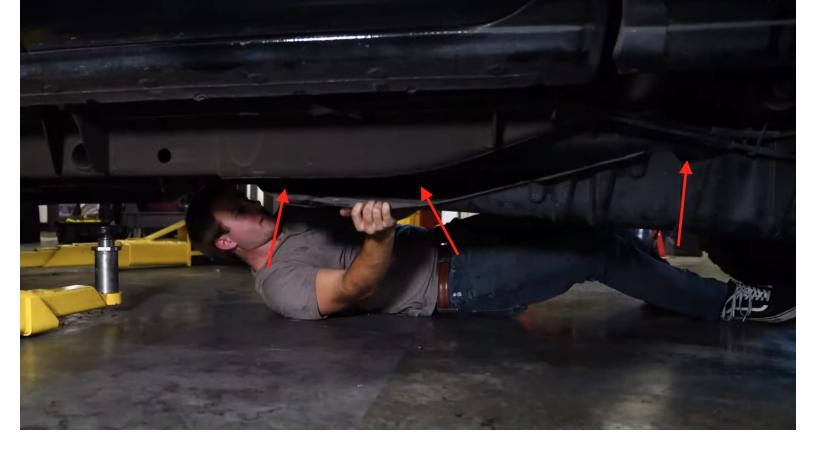
Remove the OEM skid plate if equipped. 3 bolts hold on the fuel tank skid plate. This will not be used again.
