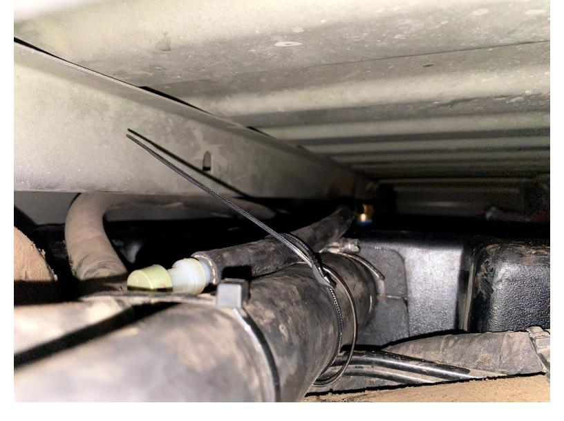
Reinstall the filler hose onto the S&B Tank and zip tie the breather line onto the filler hose.
