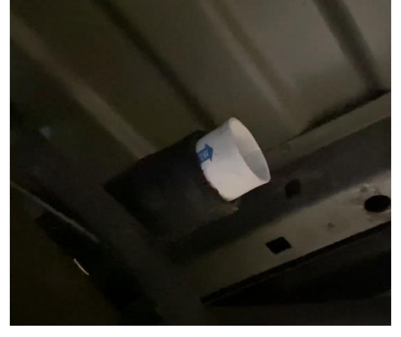
Install the white inlet check valve into the filler hose before installing the tank. The blue arrow should be pointing into the tank.
