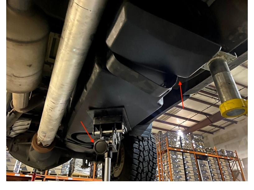
Install the S&B Straps. Start by installing the rear strap first. If you are installing this on a 2020+ truck, the included bolt can be used on the front strap to make it easier to install. Putting pressure on the underside of the front strap can help with installation.
