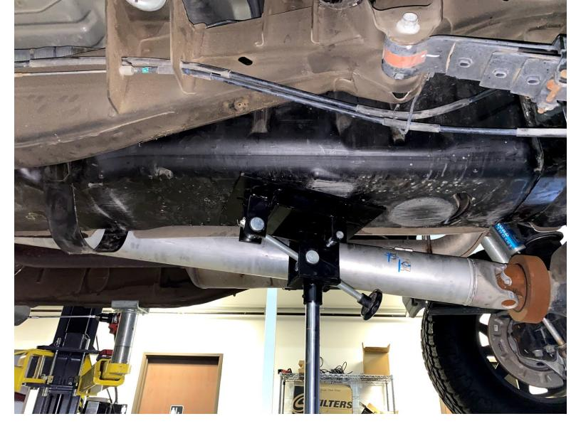
If you are doing this install on a lift, center the hydraulic jack underneath the fuel tank and raise until the jack contacts the tank. Caution: Support the tank properly as remaining fuel can slosh and cause the tank to shift. If you are doing this install on the ground, support the tank with ratchet straps, floor jack or with a partners hands while you remove the fuel tank straps.
