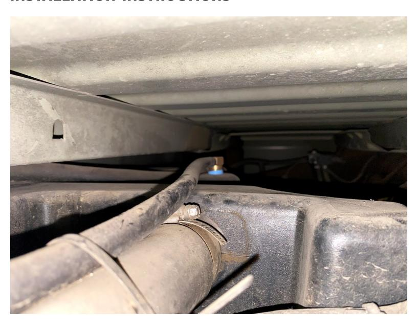
Loosen the hose clamps and remove the fill and vent lines
