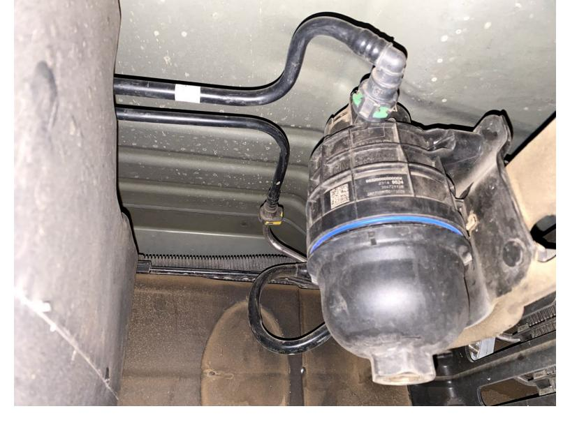
Disconnect and remove the return and feed fuel connectors.
