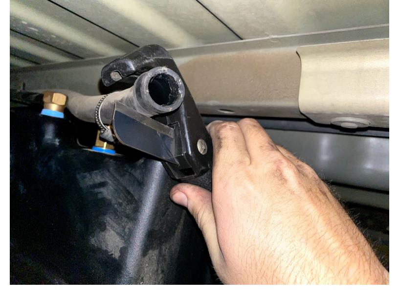
The vent hose will be installed on the S&B 5/8" barb fitting. When the tank is all the way jacked up into the truck. Measure out the correct length to cut the vent hose and make the cut. Then install the vent hose onto the barb and tighten the hose clamp
