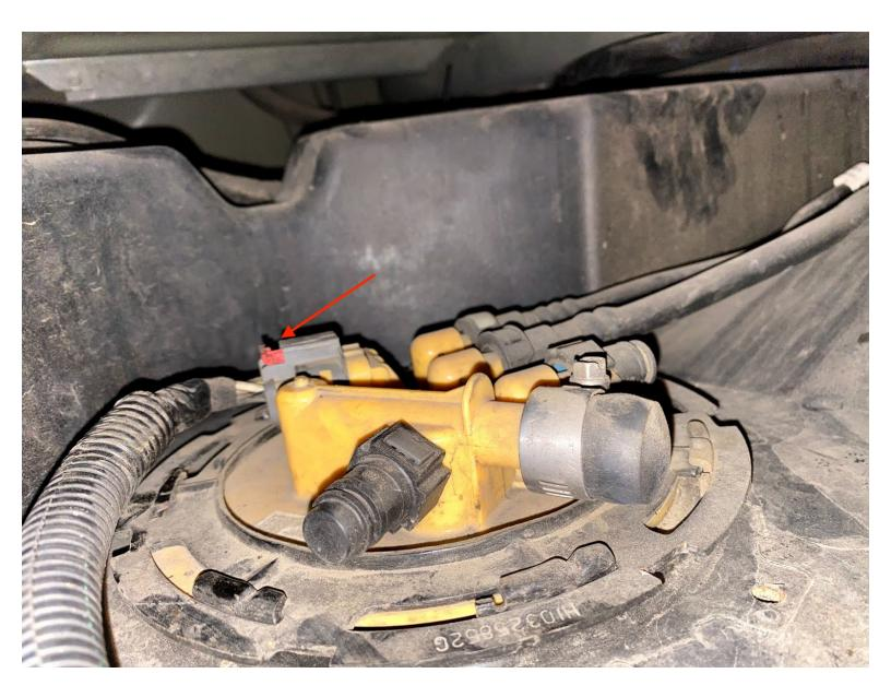
Using a precision pick or flat head screwdriver, pull out the red lock on the electrical connector. The depress the button on the top of the connector and pull the electrical connector off.
