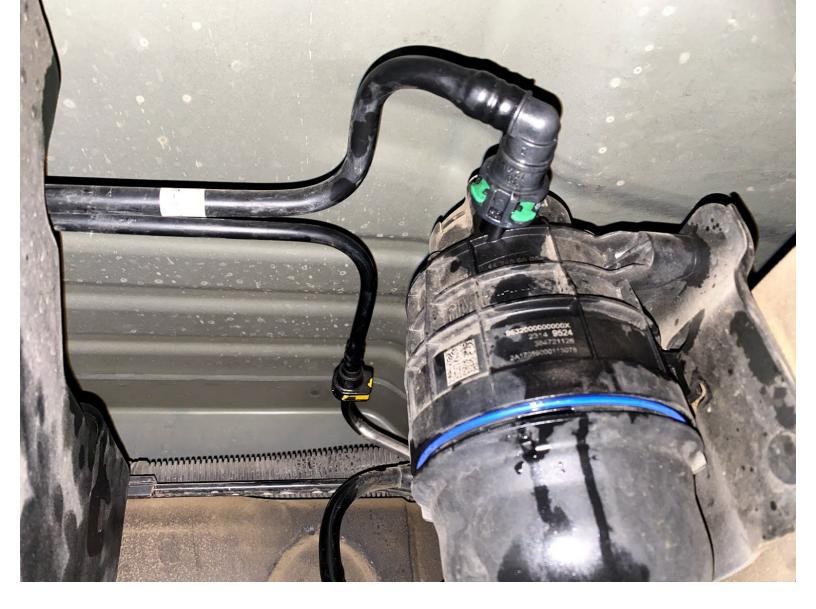
Reconnect both fuel line connectors and slide the retaining clips to the locked position. Gently attempting to separate the connectors after they are in the locked position can make sure they are connected correctly.
