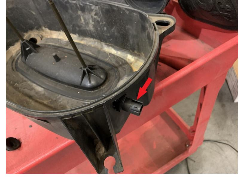
Remove the IAT sensor from the side of the stock airbox, the sensor uses a quarter turn locking pattern.
