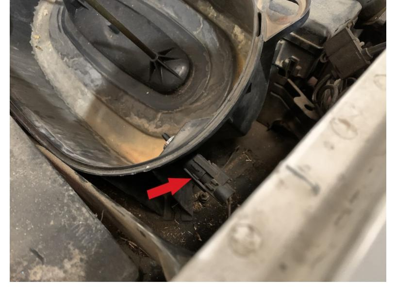
Disconnect the electrical harness at the IAT sensor on the side of the stock airbox.
