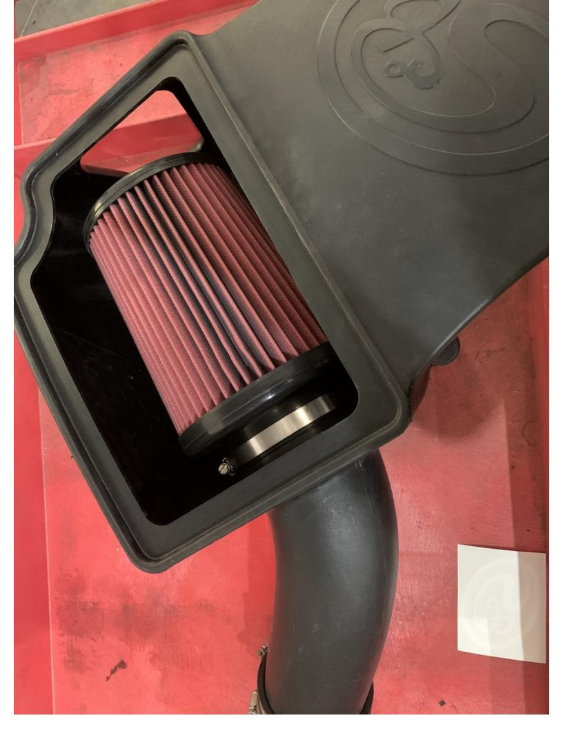
Install the Air Filter (C) loosely onto the Intake Tube (D).
