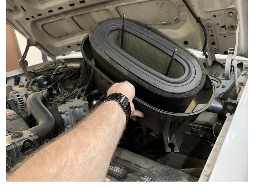
Pull up to remove the stock airbox.
