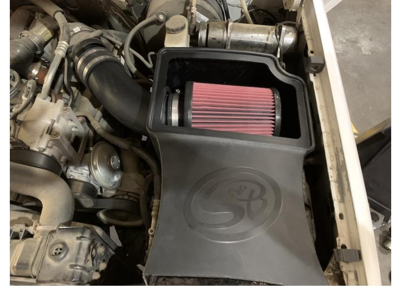
Align the Airbox Grommets with the engine bay prongs and push down on the assembly until the engine bay prongs are fully seated in the two Grommets (M).
