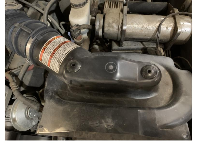
Remove the 2 fasteners on the stock airbox lid.
