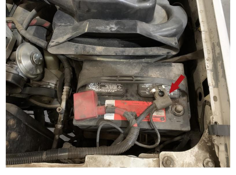
With the ignition switched off and the parking brake set, disconnect the negative battery cable on the drivers side.
