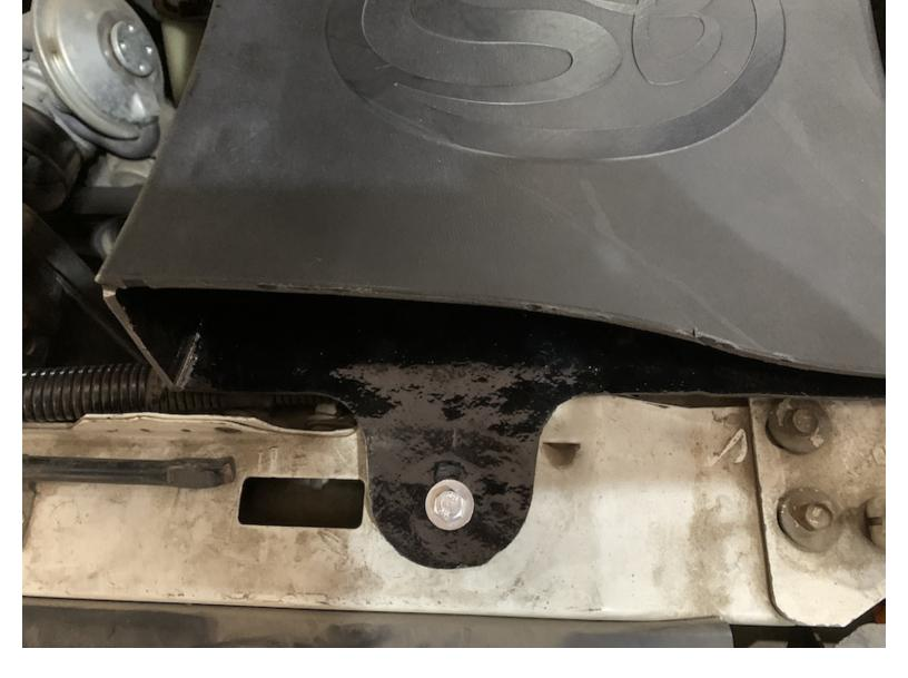
Secure the scoop to the vehicle using the M6 Bolt (K) and M6 Washer (L).
