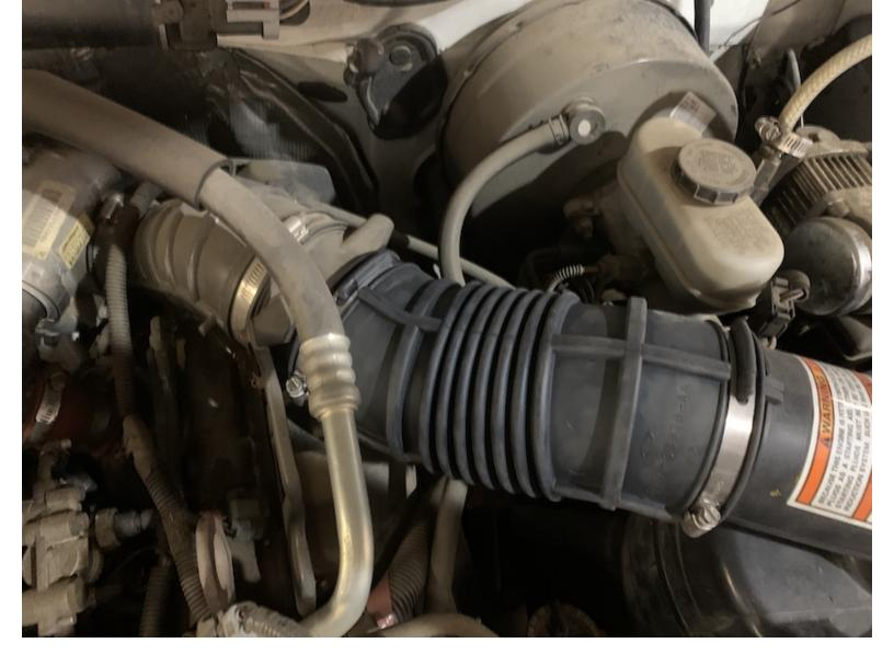
Loosen the hose clamp at the baffle.
