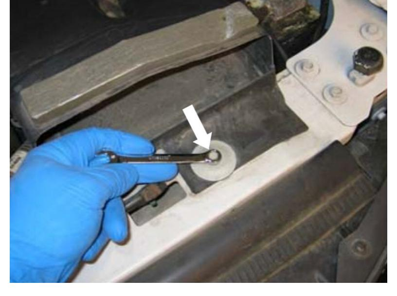
Remove the bolt and washer from the stock intake scoop. Then remove the scoop from the vehicle.
