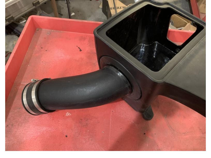
Push the Intake Tube (D) through the Tube Seal (B) until the stop bead meets up with the Tube Seal (B).
