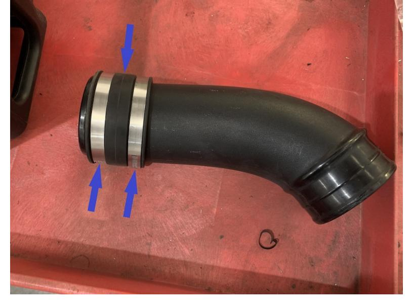
Slide the Coupler (E) and loose Hose Clamps (J) onto the Intake Tube (D) until the end of the Coupler (E) meets up with the end of the Intake Tube (D).
