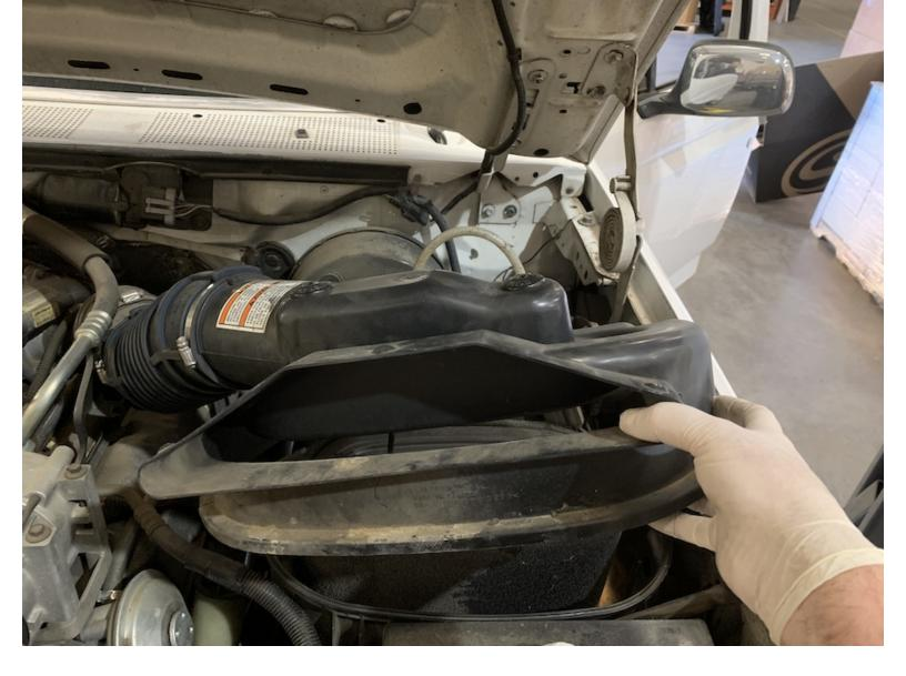
Remove the stock airbox lid and tube, then remove the stock air filter.
