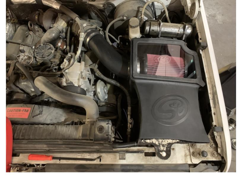
Press the lid assembly into the box opening until it snaps into place. Inspect your installation, make sure the kit is properly positioned and all fasteners are secured. Keep all stock parts in case you would ever need to reinstall the stock intake assembly. Affix the ID label near the intake kit.
