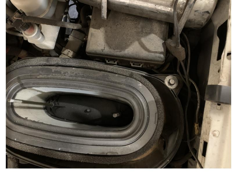
Remove the stock airbox mounting nut and washer.
