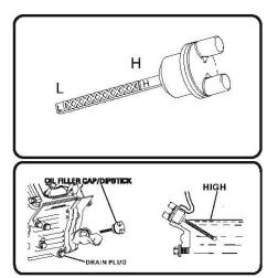
5.Replace oil fill cap/dipstick and fully tighten. 6.Reinstall maintenance cover and tighten screws. 7.Oil Level should be checked prior to each use or at least 8 hours or operation. Keep oil level maintained.
