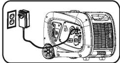
There is a light on the charger. This light will remain red until the battery get charged and then it will be changed to green. The charger won't charge the battery or will stop charging when the light is green to prevent any damage to battery and generator.
